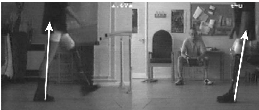
Fig. 9. Ground reaction at heel contact, one of the critical phases when stance support is required, the support provided by the knee is clearly visible on the right. The sound side loading prior to heel contact is also shown on the left for comparison.
